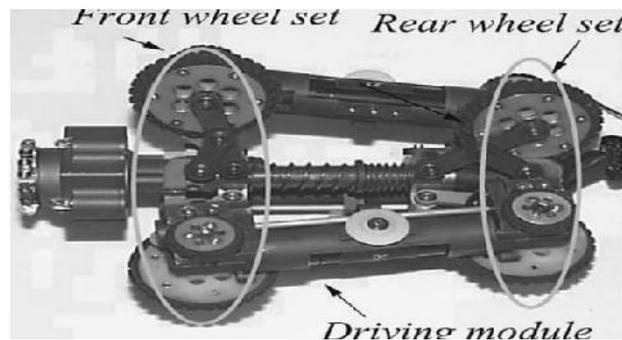
**Figure 5: Wheel Type Inspection Model [38].**
