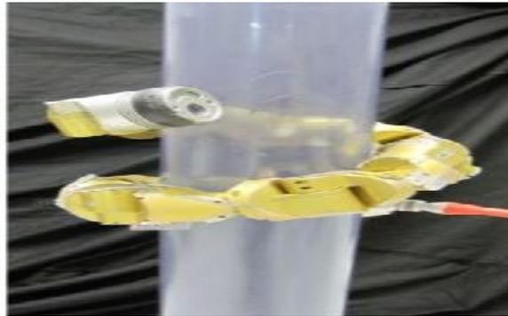
**Figure 9: Snake Type Inspection Model [65]**
