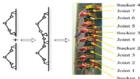
**Figure 10: Inchworm Type Inspection Model [72].**
