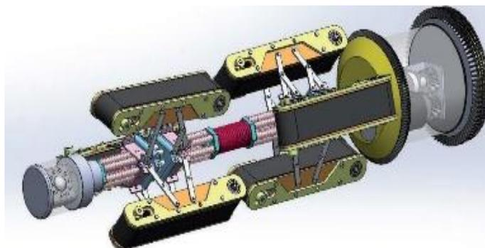
**Figure 6: Track Type Inspection Model [41].**
